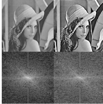
Figure 14. The original image with its FT and the sharpened image with its FT
