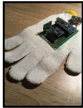
Figure 15: The transmitter unit fitted on the glove [15]
