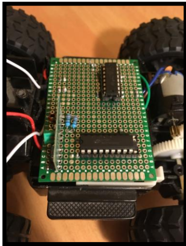
Figure 14: The receiver unit fitted on the vehicle [15]
