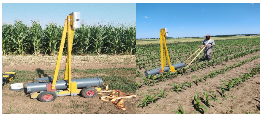
Figure 4. EM38 electromagnetic induction sensor mounted on a metal-free sledge during field measurements.
