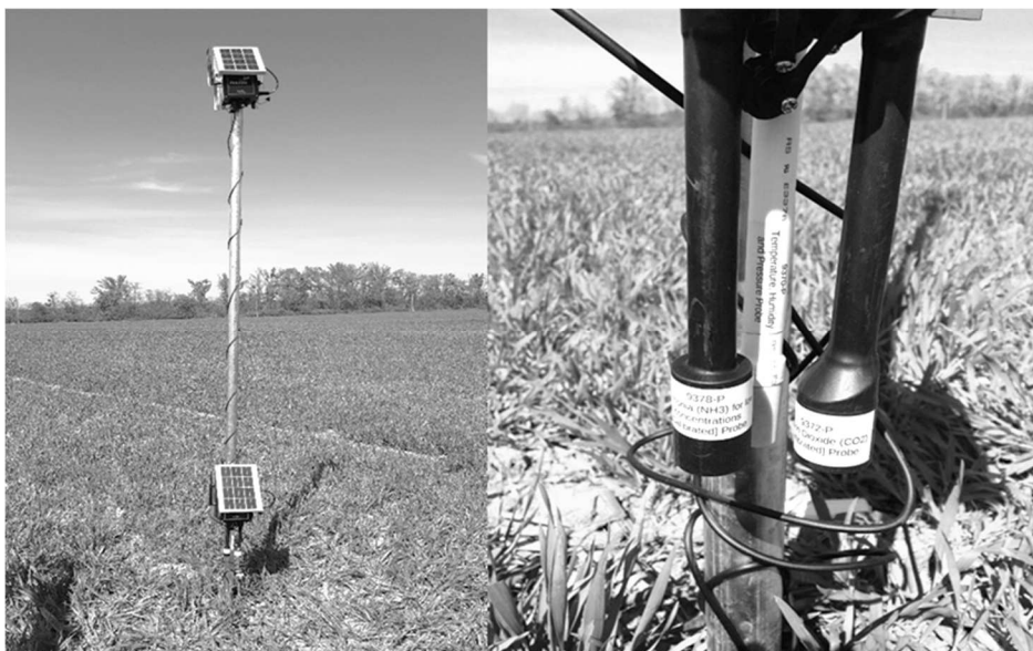
Figure 1. Ammonia and carbon dioxide sensor placed in a winter wheat crop
