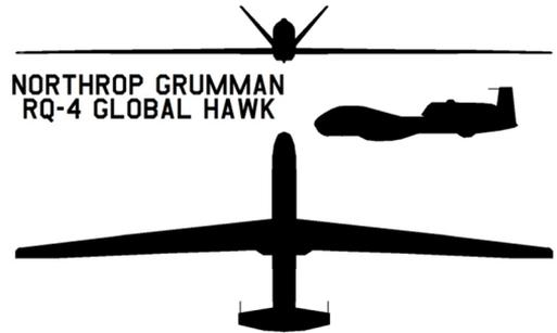
Fig. 3. Northrop Grumman RQ-4 Global Hawk Block 30 HALE UAV. Source: [http://fc05.deviantart.net/fs47/f/2009/185/9/2/Northrop\\_RQ\\_4\\_Global\\_Hawk\\_by\\_bagera3005.png](http://fc05.deviantart.net/fs47/f/2009/185/9/2/Northrop_RQ_4_Global_Hawk_by_bagera3005.png)
