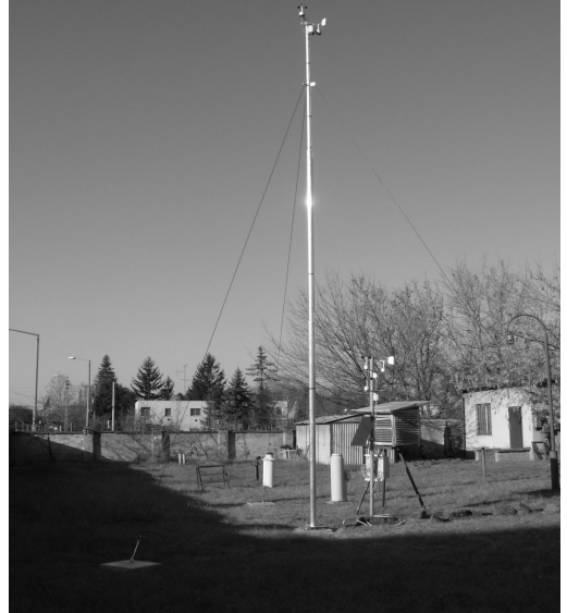
Fig. 6. The new automatic urban climate station at the Meteorological Observatory of the University of Debrecen (Source: photos of the author)
