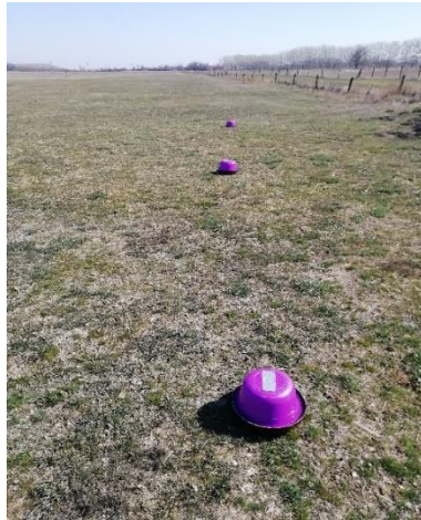
Figure 1: Frames and vessels used to measure carbon dioxide emissions Source: Own photo(1)
