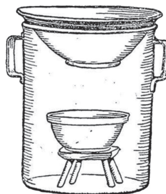
Figure 1. Primitive pálinka distillery unit
