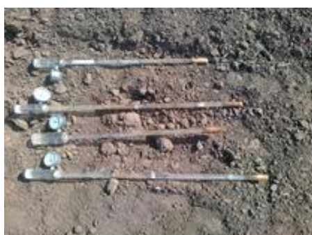
Figure 3. Soil moisture sensors arranged in parallel prior to installation in the field
