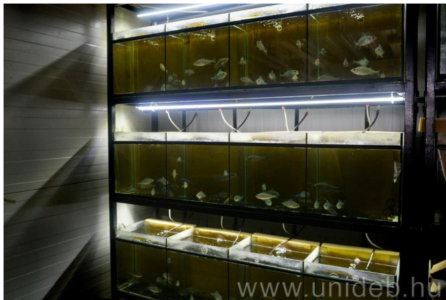
Figure 1: The experimental modular recirculating aquarium system
