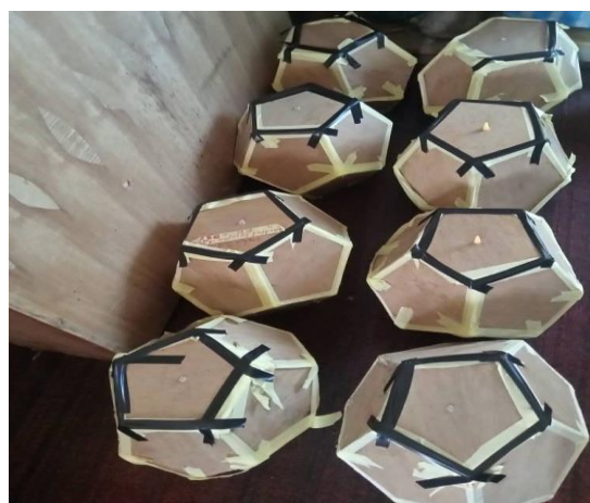
Figure 1. The picture of sealed Dodecahedron Pyramidal Shapes with thermometer and hygrometer devices placed inside for measurement of temperature and relative humidity.
