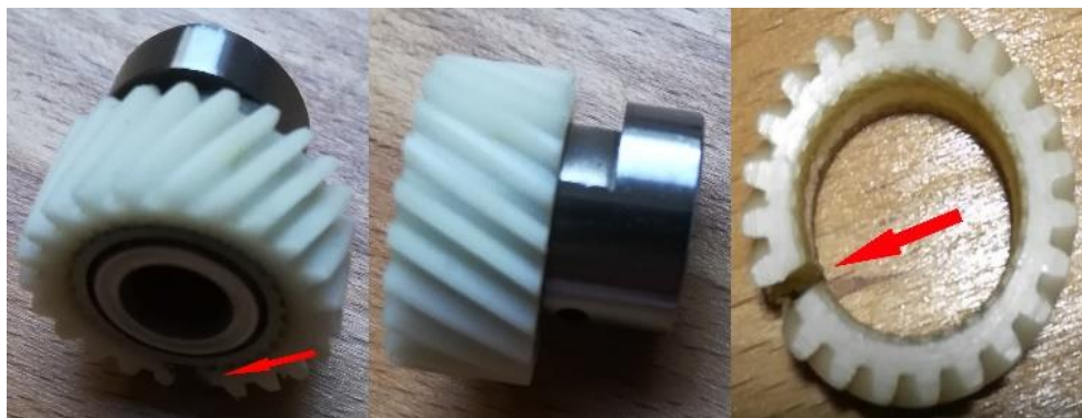
Figure 4. Broken section (shown by arrows)
