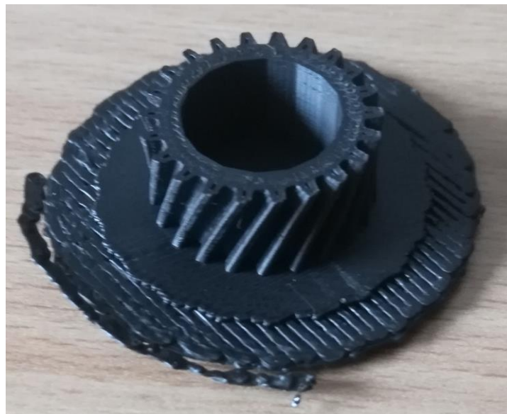
Figure 9. Finished part attached to the raft.
