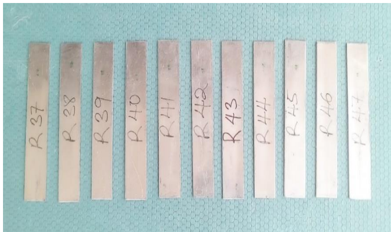
Figure 3. Samples of AA7075 thin plate after preparation
