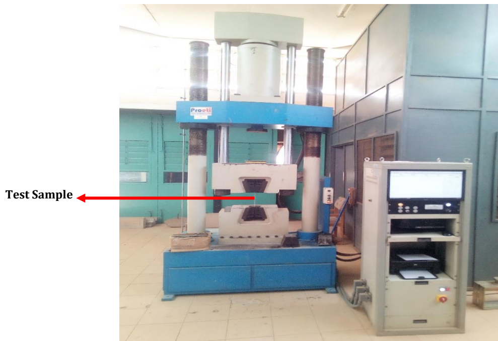
Figure 4. Experimental set-up for the tensile test
