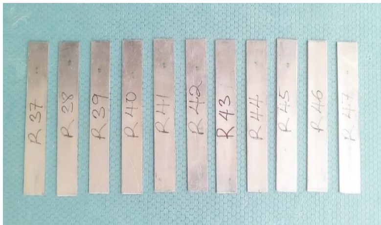
Figure 3. Samples of AA7075 thin plate after preparation
