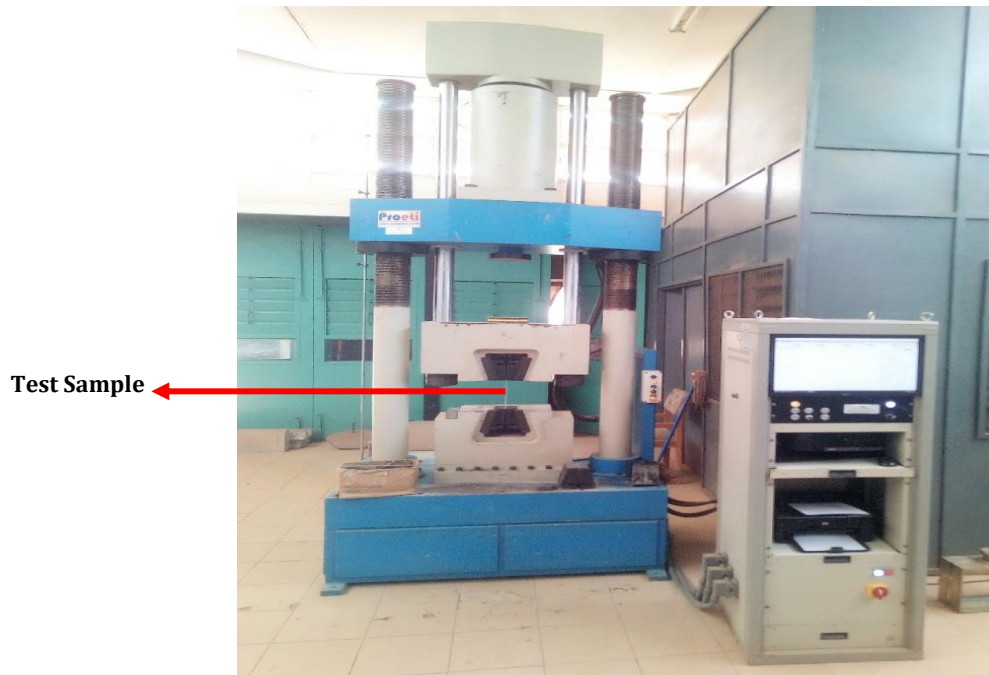
Figure 4. Experimental set-up for the tensile test
