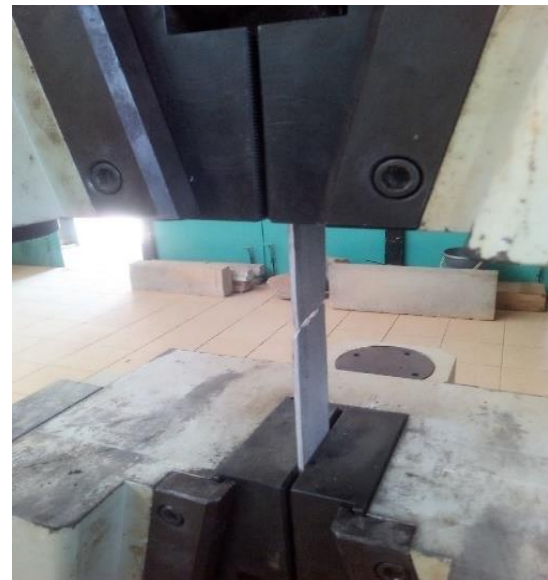
(b) A fractured sample after the test
