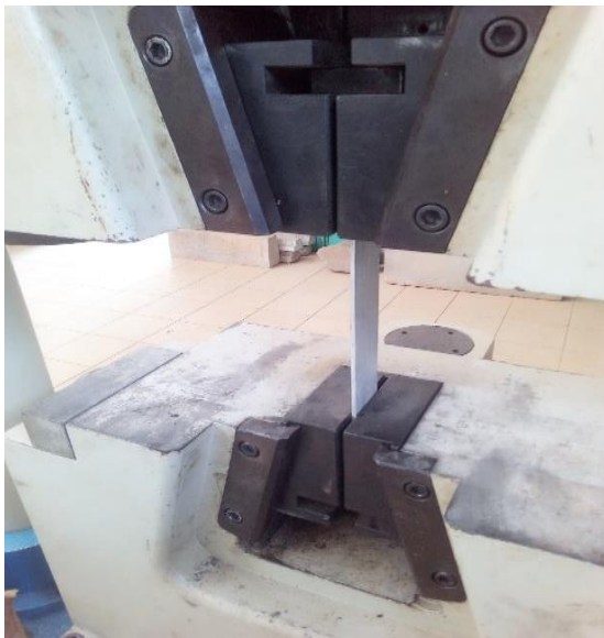
Figure 5. (a) Unfractured sample before the test
