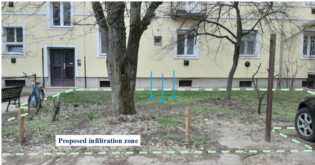
Figure 18. Proposed stormwater infiltration zone as a rain garden
