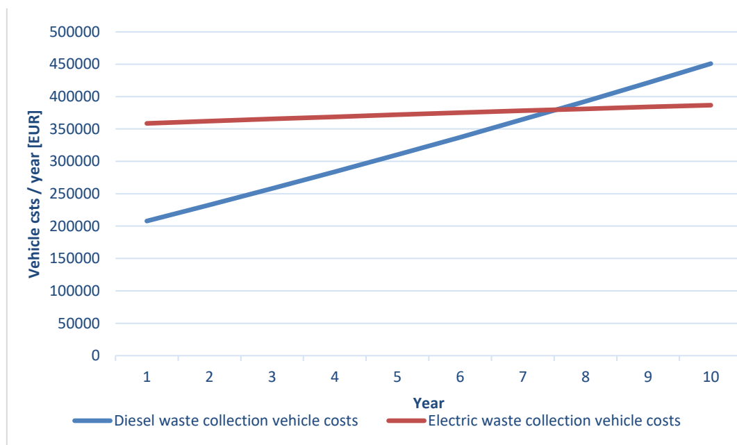
Figure 2. Changes in the cost of diesel and electric waste collection vehicles over 10 years
