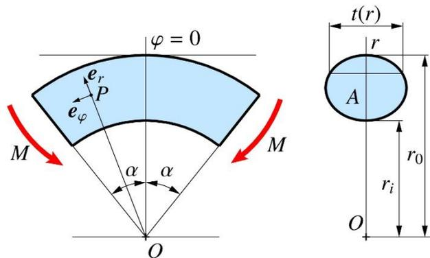
Figure 1. Curved beam loaded by bending moment.
