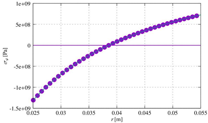
Figure 3. The plot of the hoop stress  $\sigma_\varphi$  as a function of  $r$ .
