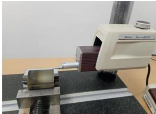
Figure 3. Measurement of surface roughness parameters R_a and R_z of samples made by electroerosive technology.
